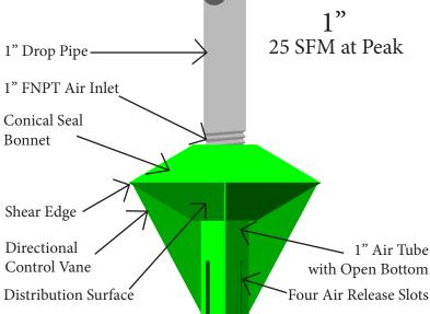
Shear tubes and draft tubes in combination with the G-O Diffuser can provide excellent mixing and efficient aeration of deeper basins while maintaining lower blower pressure requirements. The G-O Diffuser is particularly suitable for grit basins, digesters and other high solids application.
