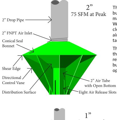
The G-O Diffuser is a single-drop medium bubble aeration diffuser that is truly no-clog, maintenance free and continuously efficient. With no orificing below the water surface clogging is eliminated due to the free flow of air through the drop pipe. Providing superior tank mixing with lower air flows required.
